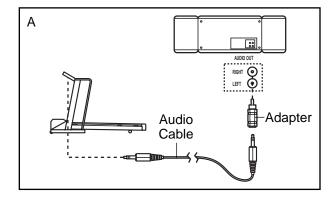
B. Plug one end of the audio cable into the jack beneath the console. Plug the other end of the cable into the LINE OUT jack on your stereo.
